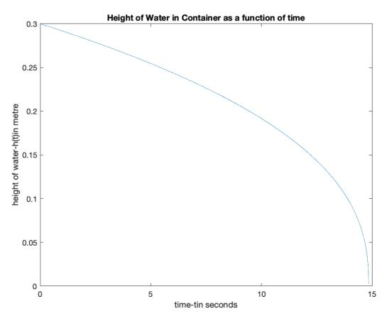
The graph shows linear declination in height of water in container with time. To check the validity we can observe that the graph ends at  $\tau = 14.8461$  s which is the same as the value of  $\tau$  calculated so it stands valid.
